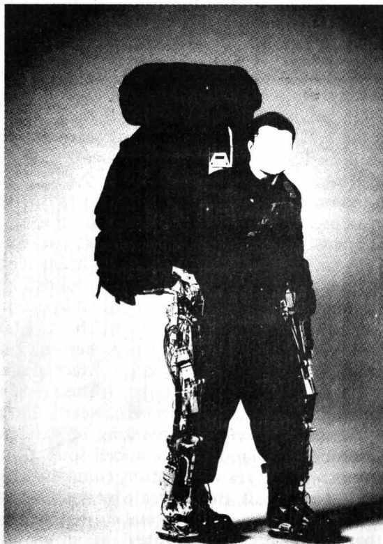
The Berkeley Lower Extremity Exoskeleton is now ready for production. If you liked those pesky Marines before, you'll love version 2.0.
