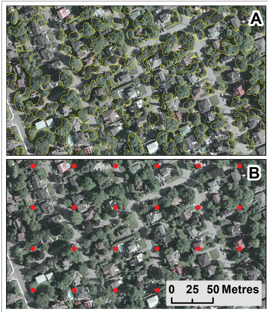
Fig. 6.1. Commonly used canopy cover analysis methods including (A) manual digitizing of canopy cover and (B) point-based sampling.
