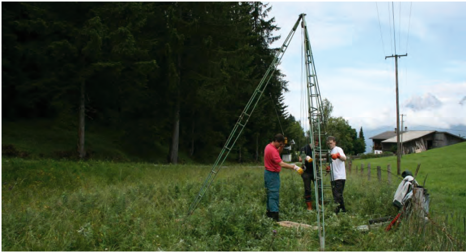
Figure 1: Coring (Geonor piston corer) at the Kogelmoos fen (Courtesy of the author)
